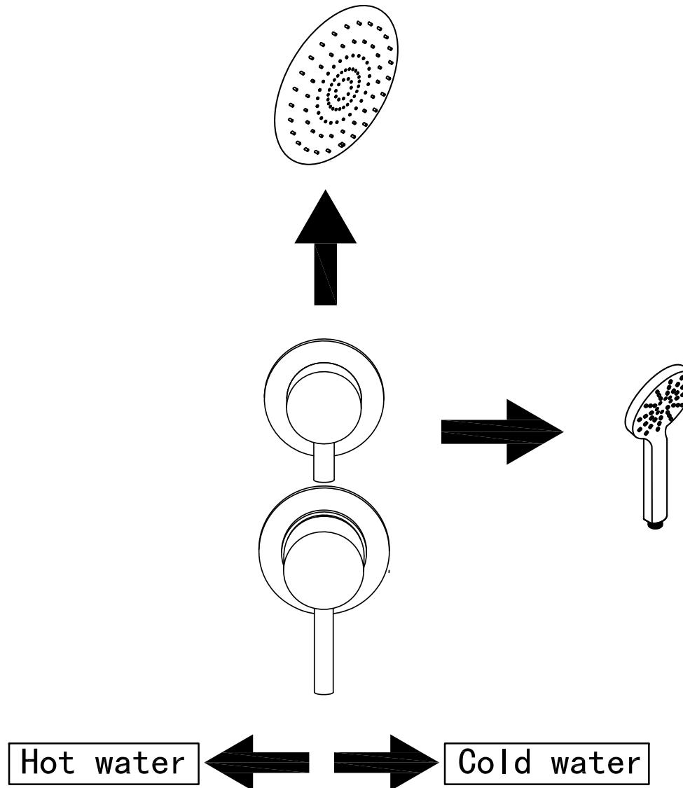
ENG: Ideal water function for proper functioning of the mixer and its functions : 8 Bar to 16 Bar
