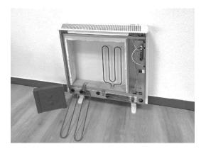
9. - Place the storage bricks carefully, with the flat side facing the back of the heater. Arrange two row levels of bricks.
