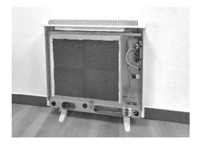
II. Replace the inner front panel. If the bricks have been fitted correctly you will have no difficulty in replacing the panel. Make sure the bottom edge of the inner panel is inside the front lip of the heater. Please see below:
